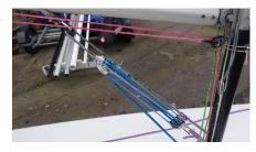
Tighten the mainsheet horse. Multiple purchase between the two eyelets works best. This allows the boom to set in line with the aft corner. The boom needs to be set at the correct angle to the centreboard upwind. If the horse is slack the boom will move to the centre of the boat.
