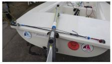
Mark the outhaul position. I add tape to the boom so I can set the position the same each time. The gap between the boom and sail should be around 4 finger widths. My outhaul sets to the forward black mark (as in the photo) upwind, the green and yellow on a reach and rear black mark downwind.
