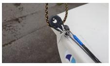
Strap down the clew of the sail separately. I have a rope and bobble secured to the boom. This holds the sail down lower to allow you to bend the mast more. This is an extra step to rig.
